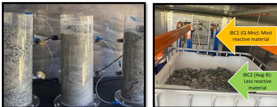
Fig. 9. Design of Columns and IBCs container
