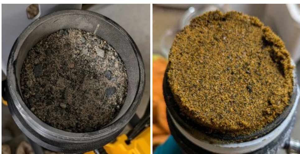
Fig 3: Filter sand (a) initial conditions and (b) conditions after 97 days
