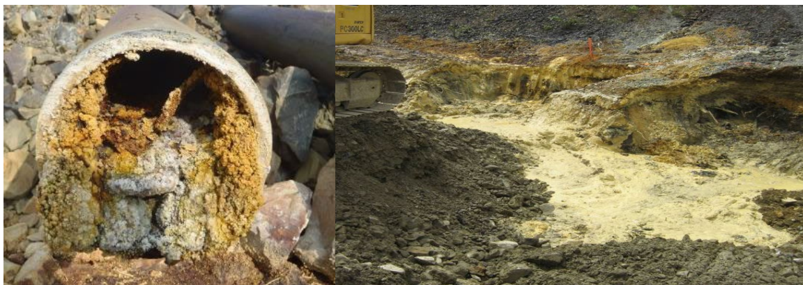
Fig 1. Examples of clogged pathways from TSFs: Drain pipe (L) and seepage zone (R)
