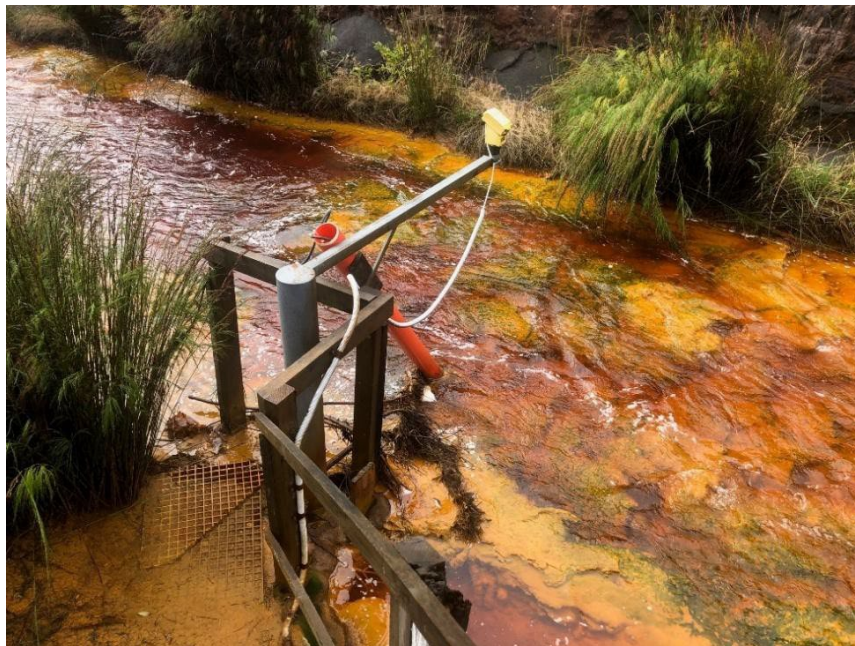
Fig.2. Image of Vesi™ sensor technology installed in AMD creek during the trial
