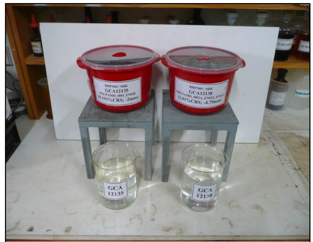
Fig. 3. Mass of reacted dewatered solids (left) and extracted water (right)
