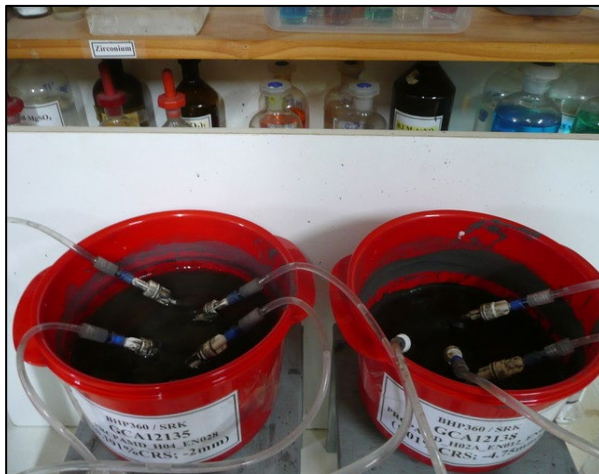
Fig. 2. Porewater extraction using Rhizon® pore water samplers
