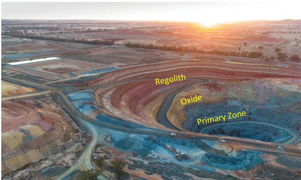
Figure 9: Wyoming One Pit showing cover and depth of oxidation (Source Alkane Resources)
