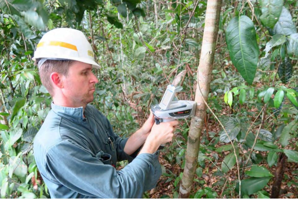
Using handheld XRF to measure concentrations of nickel in a hyperaccumulator tree in the field in Indonesia.
