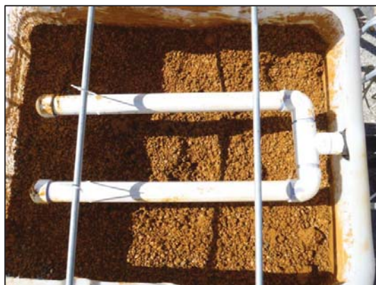
Fig. 2. Adsorption chamber (on left) and bioreactor (on right) prior to being filled with water
