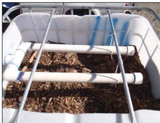
Fig. 2. Adsorption chamber (on left) and bioreactor (on right) prior to being filled with water
