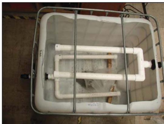
Fig. 1. Adsorption chamber prior to being filled with treatment medium
