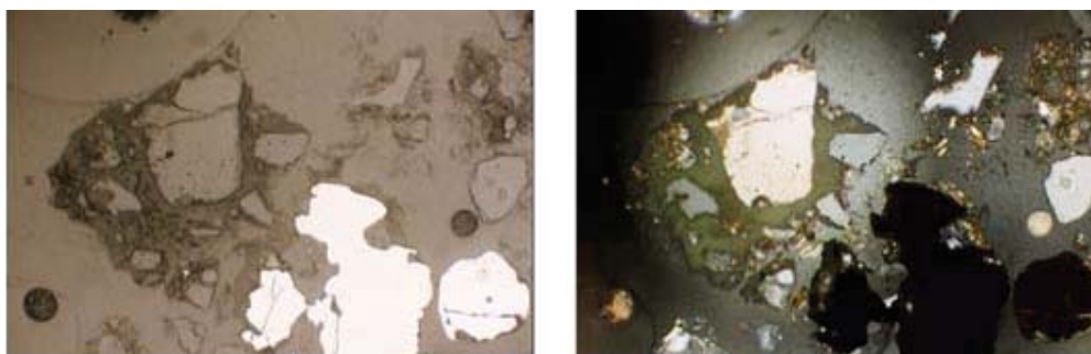
Fig. 3. Sample obtained from the Keystone dump at BCM showing a plain reflected light image (left) and an internal reflected image (right) of the same field (1.3 mm in width). On the left of the two images is a pyrite clast that is contained within a jarositic cement (greenish colouration on the right image).
