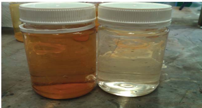
Fig. 2. AMD water before and after treatment by pilot plant.
