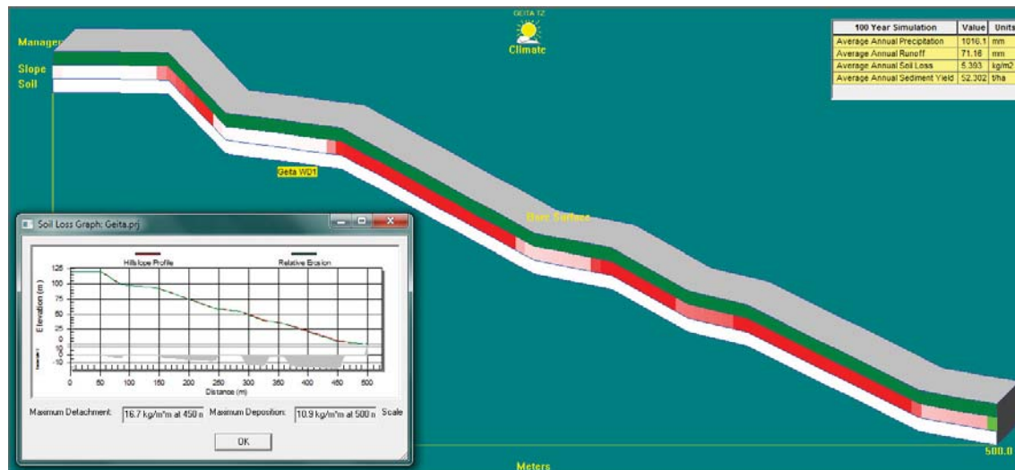
Fig. 6. Results of WEPP modelling for the existing WD1 embankment profile.
