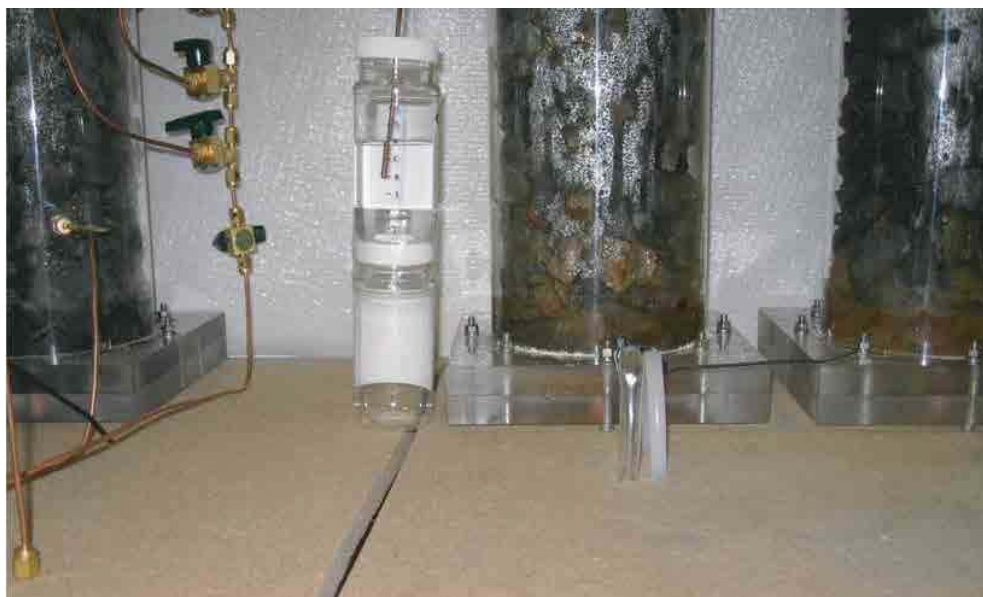
Fig. 8. The reddish oxidation product concentration in columns 2 and 3 (right) and no precipitation in column 1 (with IGM - left) in the same time frame.
